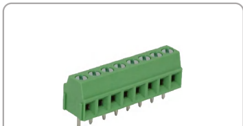
EBHS381 Pitch 3.81mm Poles 2p~24p PCB screw terminal blocks, horizontal wire inlet
