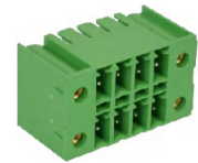
HFCH381 Pitch 3.81mm Poles 2*2p~2*24p Double-level Header with threaded flange, plug-in direction parallel to the PCB
