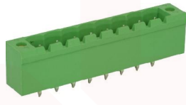
HACV500 Pitch 5.0mm Poles 2p~24p Header with threaded flange, plug-in direction vertical to the PCB
