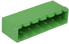
HABH500 Pitch 5.0mm Poles 2p~24p Header, plug-in direction parallel to the PCB
