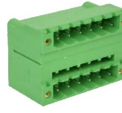
HAFH508 Pitch 5.08mm Poles 2*2p~2*24p Double-level Header with threaded flange, plug-in direction parallel to the PCB
