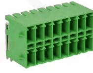
HFDH350 Pitch 3.5mm Poles 2*2p~2*24p Double-level Header, with engagement nose, plug-in direction parallel to the PCB
