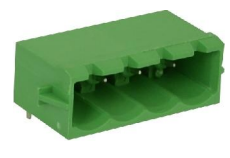
HADH508 Pitch 5.08mm Poles 2p~24p Headers with engagement nose, plug-in direction parallel to the PCB
