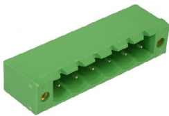
HACH508 Pitch 5.08mm Poles 2p~24p Header with threaded flange, plug-in direction parallel to the PCB
