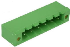
HACH500 Pitch 5.0mm Poles 2p~24p Header with threaded flange, plug-in direction parallel to the PCB
