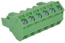
MESO508 Pitch 5.08mm Poles 2p~24p Plug-in direction 45D to the conductor axis
