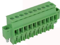
MBFR381 Pitch 3.81mm Poles 2p~24p Plug, hook on entry side, with screw flange
