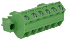
MEFO508 Pitch 5.08mm Poles 2p~24p Plug-in direction 45D to the conductor axis
